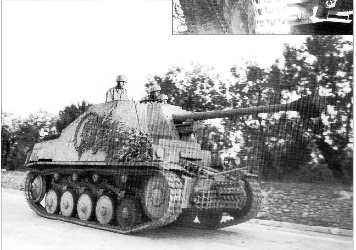
An Sd.Kfz.131 Marder II self-propelled anti-tank gun of Panzer-Artillerie-Regiment 'Hermann Göring' in Southern Italy in late 1943. Mounting the 7.5cm PaK40/2, 576 Marder II's were manufactured between June 1942 and June 1943 with another 75 converted from obsolete Pz.Kpfw.II chassis from July 1943 to March 1944. The crew has been issued with standard M38 Fallschirmjäger helmets.
