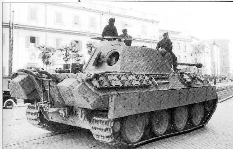
A new Panther Ausf.A from I./Pz.Rgt.4 travelling with the column through Rome in February 1944. It is fitted with the early 16 bolt roadwheels that have been reinforced with 16 rivets. Note the boarding ladder suspended from the cross bar between the exhaust pipes.
