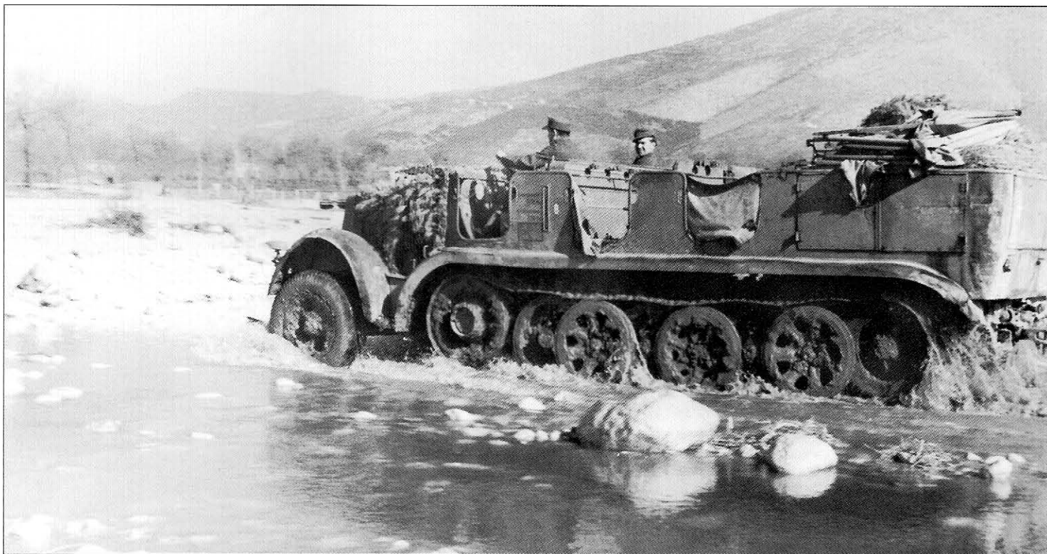
An Sd.Kfz. 7 8t half-track prime-mover fords a shallow stream in Central Italy. The shipping stencil can be seen painted in black on the side panel behind the driver along with a white '8'. They were normally employed for towing heavy artillery pieces such as the 15cm sFH18 and the 8.8cm FlaK guns. Over 12,000 units were manufactured between 1934 and 1944.
