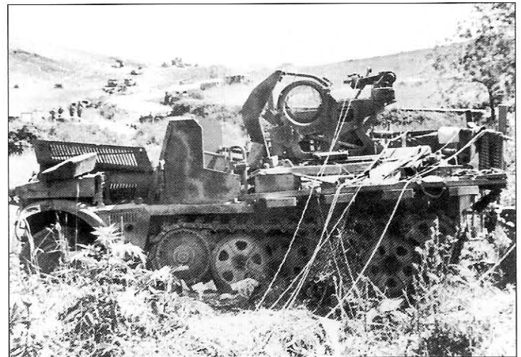
An Sd.Kfz.10/5 abandoned near Rome in June 1944. It is armed with the 2cm FlaK38 anti-aircraft gun and has been fitted with a light armored shield around the driver's compartment. This one is painted overall dark yellow with a camouflage scheme of brown and green patches.
