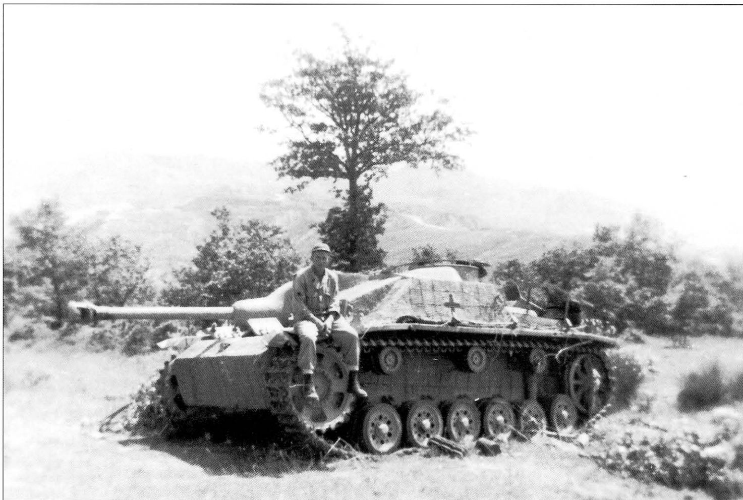
An American soldier sits on a knocked out StuG.III Ausf.G. It features the waffle pattern Zimmerit coating applied at the Alkett plant between September 1943 and September 1944. It is also fitted with the 'topfblende' cast gun mantlet and the shot deflector in front of the commander's cupola. Steel return rollers were introduced in November 1943, however rubber tired rollers continued in use until stocks were used up.
