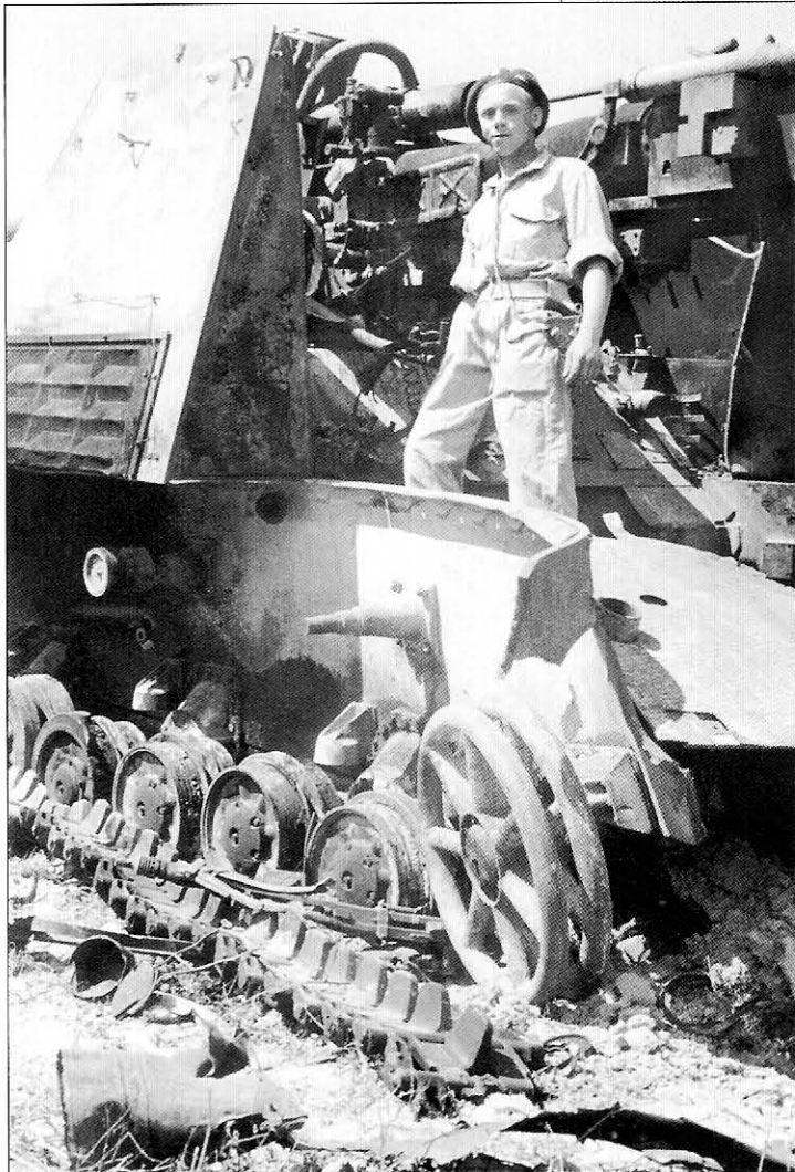
An Sd.Kfz.10/5 abandoned near Rome in June 1944. It is armed with the 2cm FlaK38 anti-aircraft gun and has been fitted with a light armored shield around the driver's compartment. This one is painted overall dark yellow with a camouflage scheme of brown and green patches.
