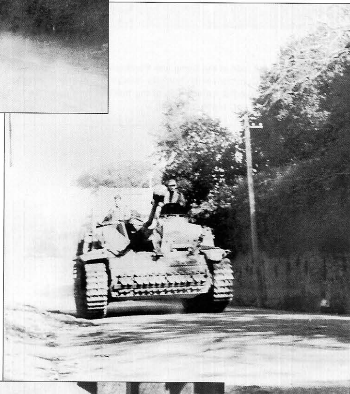
A damaged early Jagdpanzer IV awaits a recovery vehicle to tow it to the workshops. The transmission has probably seized up and so both tracks have been shortened and linked together bypassing the drive sprocket. The early Jagdpanzer IV mounted the 7.5cm PaK39/L48 gun, some of which were fitted with a muzzle brake like this one. From January to November 1944, a total of 769 of these purpose built Panzerjäger were built and saw their first action with Panzer-Division 'Hermann Göring' in the spring of 1944.
