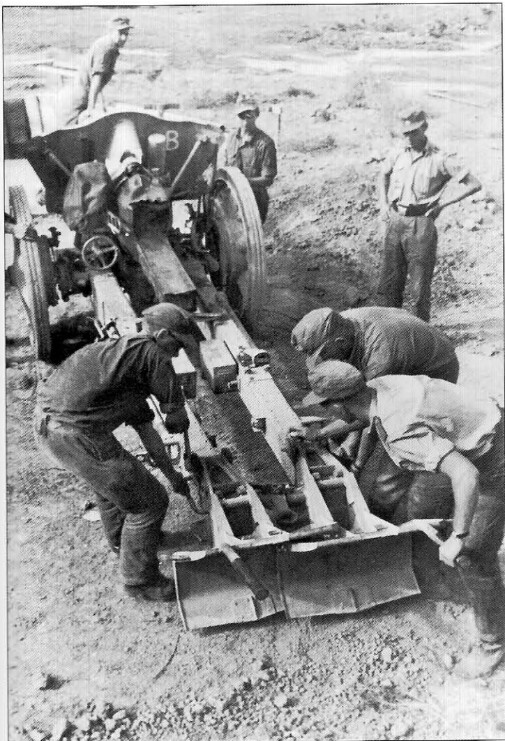
A 10.5cm leFH18 or leFH18M (M – mundungbremse – muzzle brake) is maneuvered into a prepared gun emplacement. One of the crew has added his weight on end of the gun barrel to help balance the heavy gun trails as they are opened up. Unfortunately, he has also blocked the view of the muzzle, which would indicate if the piece were fitted with a muzzle brake or not. The leFH18 was the backbone of the German artillery and served from 1935 to 1945. It fired a 14.8kg high explosive shell and had a maximum range of 10675m.
