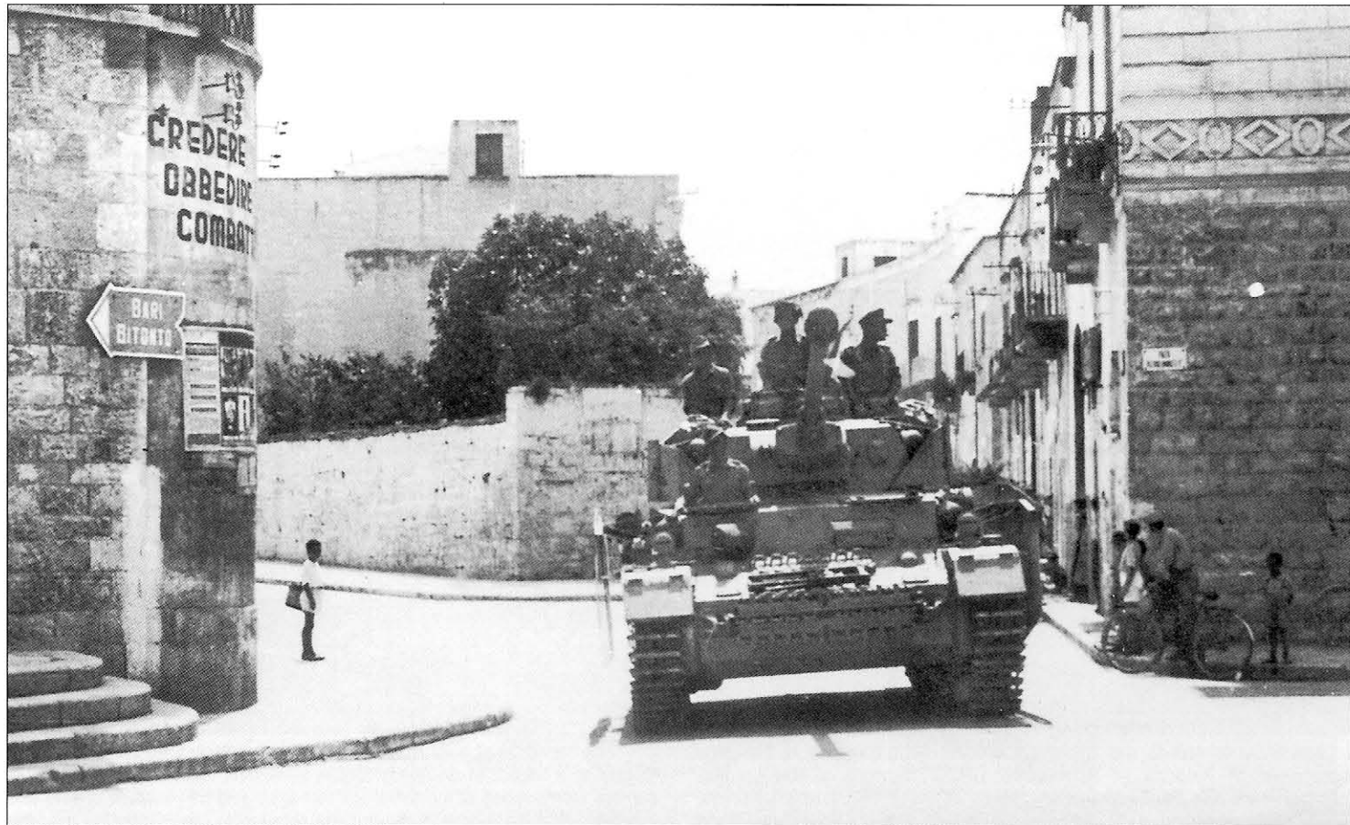
A column of new Pz.Kpfw.IV Ausf.G move through an Italian town near the Adriatic coast. The Panzer is finished in overall dark yellow and the only visible marking is the black Balkenkreuz painted on the side of the turret skirt armor. Note the dust covers installed on the muzzle brake and hull mounted machine gun. They are probably from 16.Panzer-Division, the only unit equipped with Pz.Kpfw.IV in Southern Italy at the time.
