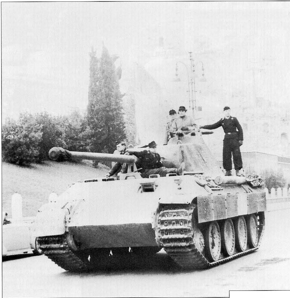
A column of Panthers from I.Abteilung/Panzer-Regiment 4 travel along the Via dei Fori Imperiali towards the Colosseum in February 1944. This is an early Panther Ausf.A and features the 'letterbox' machine gun port on the glacis. The tactical number '215' is painted in red with a white outline on the side of the turret. The vehicle appears to be painted in a severely weathered and dirty overall dark yellow over a rough coating of Zimmerit.
