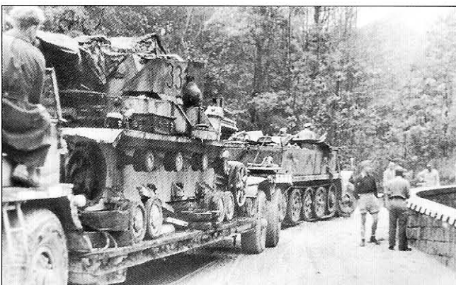
An Sd.Kfz.9 heavy half-track prime mover tries to negotiate a tight curve on an Italian mountain road in late 1943. The 18t Famo is towing an Sd.Ah.116 trailer carrying a severely battered Pz.Kpfw.IV Ausf.G from Pz.Rgt. 'Hermann Göring' on it. The Pz.Kpfw.IV Ausf.G is painted in overall dark yellow with a patchy green camouflage pattern and a three digit tactical number, '331', painted in red with a white outline on the side of the turret skirt armor. The Famo is also painted in overall dark yellow but has a wide green horizontal zig-zag camouflage stripe painted on the cargo box.
