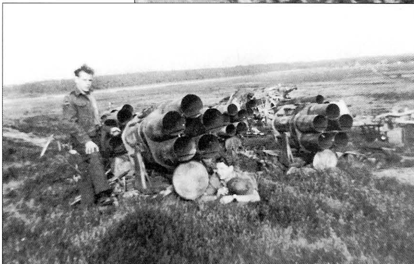
Two soldiers from the Calgary Tanks (14th Armoured Regiment) inspect the remains of a captured battery of 21cm NbW41 rocket launchers. The rockets were fired electrically in sequence from each tube in order to avoid upsetting the unit.
