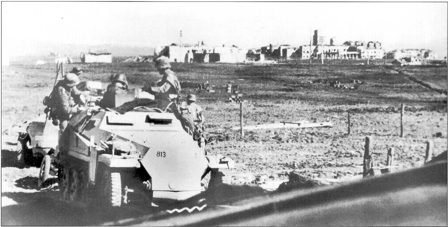
German troops clamber aboard a column of Sd.Kfz.250 half-tracks on the outskirts of an Italian town. This vehicle appears to be new and is painted in overall dark yellow. It also has the additional sheet metal stowage lockers along each side fitted to some vehicles. The numbers on the front are unusual and are not duplicated on the following vehicle. Both have the standard Wehrmacht registration number painted on front, though the glare from the sun makes the one on the front vehicle almost invisible.
