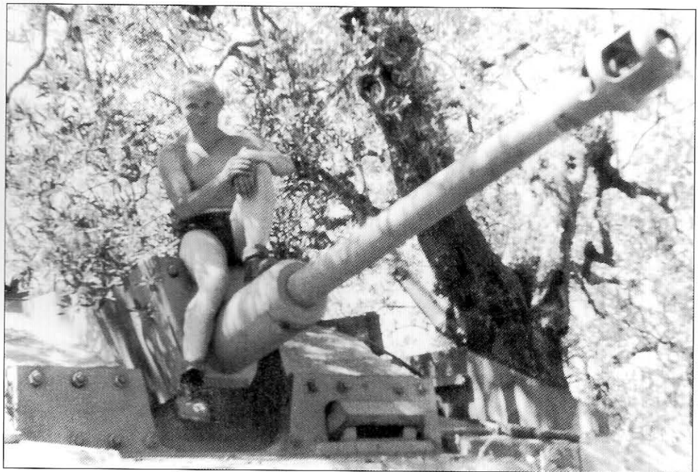
A crewman from the same unit poses on the mantlet of his StuG.III Ausf.G. This vehicle is also one of those manufactured on the chassis of a Pz.Kpfw.III Ausf.M as indicated by the longer deflector in front of the driver's visor and the wide gap between the bolts that fasten the 30mm supplemental armor above the driver's visor.
