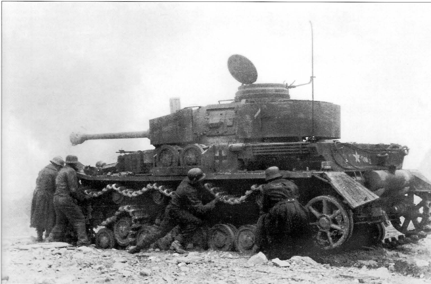
The crew of this Pz.Kpfw.IV Ausf.H struggle to replace a damaged track. It is likely that the track simply broke since there appears to be no mine damage to the suspension. They have their work cut out for them as one end of the track has wound itself up between the second and third roadwheel. The white star marking on the rear plate indicates this vehicle is from 15.Panzer-Grenadier-Division. Beside it is a white rhomboid, the tactical sign for a Panzer unit followed by the number '2', indicating the company to which the vehicle is assigned.
