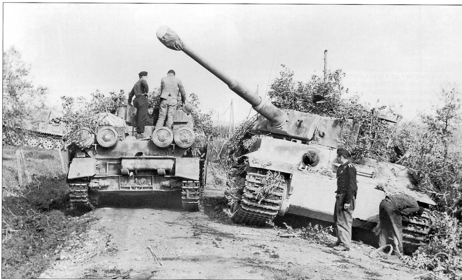
Another Sturmpanzer IV from Sturmpanzer-Abteilung 216 passes a disabled Tiger I Ausf.E from s.Pz.Abt.508 near Anzio. This one was built on the chassis of a Pz.Kpfw.IV Ausf.G. The exhaust port for the turret traverse muffler has been plated over and it is fitted with the early plated covers over the fighting compartment ventilators as can be seen to the right of the crewman standing on the engine deck. In the background, an Sd.Kfz.9 Famo heavy half-track prime-mover is waiting to move in and recover the Tiger I.
