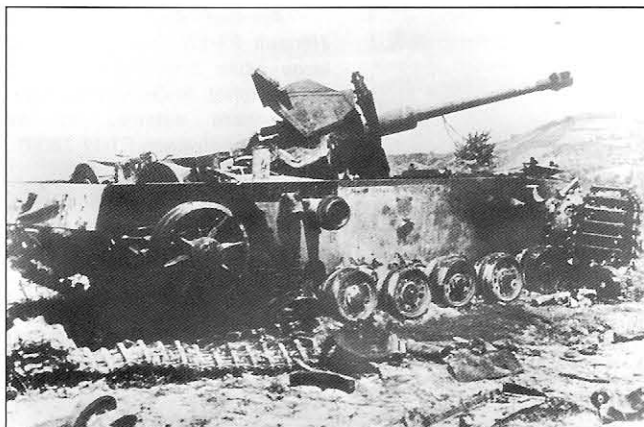
The remains of a totally destroyed StuG.III Ausf.G near Bologna in the spring of 1945. This was a later production vehicle manufactured after September 1944, when Zimmerit was no longer applied. Before being knocked out, this crew had successfully destroyed six Allied vehicles as shown by the number of kill rings on the gun barrel.
