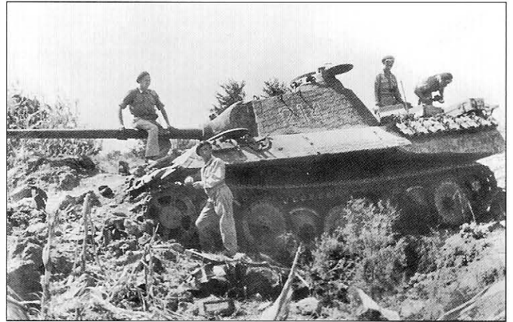
A view of the left side of the same late Panther Ausf.A from I./Pz.Rgt.4 with several British Commonwealth soldiers checking it out for souvenirs. The impact from a projectile on the side of the hull has torn away the gun cleaning rod tube and part of the tool rack.
