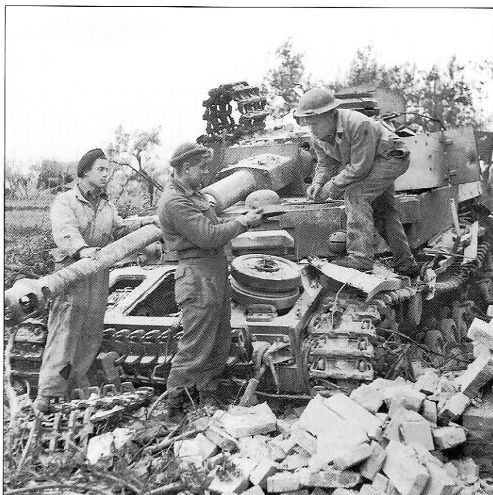
Another knocked out Pz.Kpfw.IV Ausf.G is searched for souvenirs by three soldiers from the Canadian Three Rivers Regiment (12th Armoured Regiment) in October 1943. This one has been fitted with additional 30mm armor plates that have been welded to both the superstructure and hull fronts. The curved armor shield around the final drive is missing and has probably been shot away by the impact of the round that also damaged the track. Two penetrations can also be seen in the front of the turret beside the gun mantlet. These tanks are probably from 26.Panzer-Division, which fought in this area.
