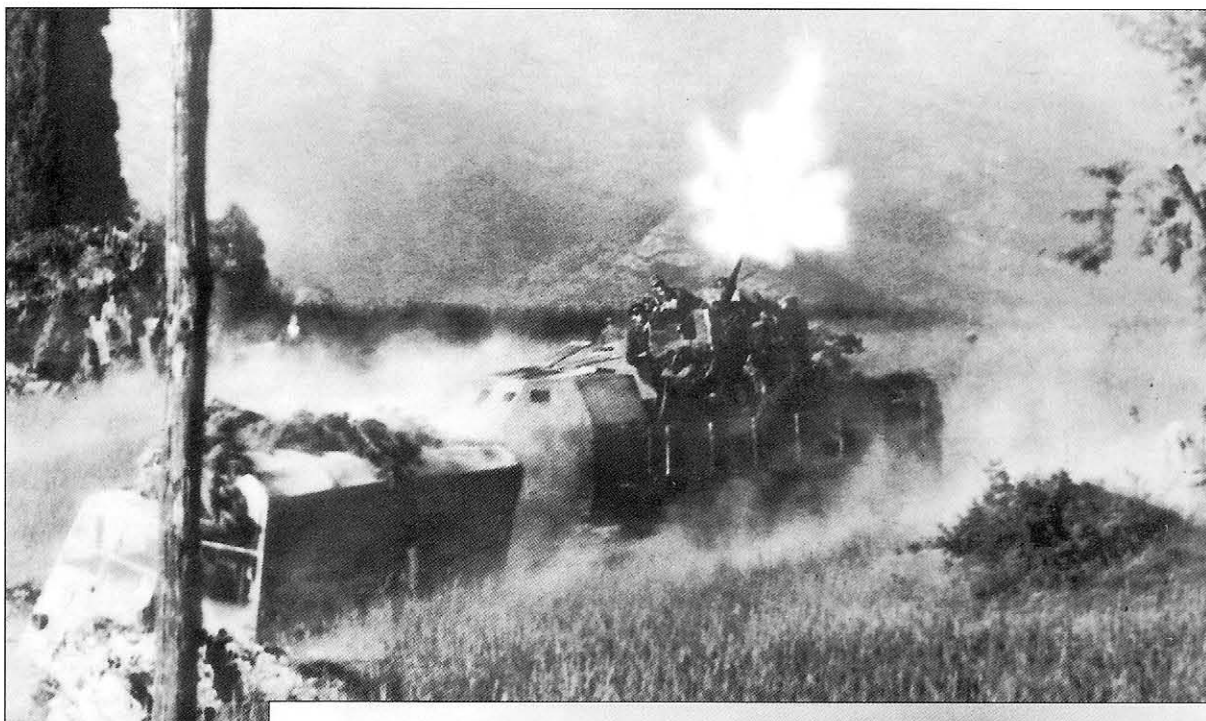
A dramatic photo of an Sd.Kfz. 7/2, mounting a 3.7cm Flak36 anti-aircraft gun, in action. This one is fitted with the light armored cab and engine compartment that began to be fitted to some vehicles in late 1943.
