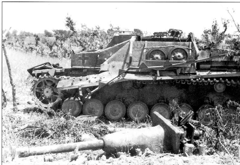
A Sturmgeschütz.IV knocked out in the Pontecorvo area near Cassino in May 1944. The StuG.IV was hurriedly developed in December 1943 to replace lost production of StuG.III after a bombing raid on the Alkett plant in November. The first 30 were completed in December 1943 and production continued until April 1945 with some 1141 built altogether. This one is from 90.Panzer-Grenadier-Division, which received 42 of these vehicles in February 1944, all of which were coated with Zimmerit.
