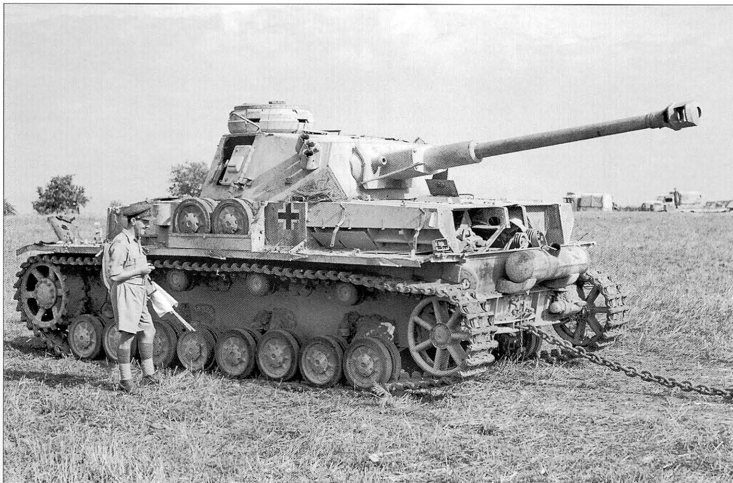
A Pz.Kpfw.IV Ausf.G from Pz.Rgt.2 of 16.Panzer-Division, knocked out in the British sector near Lucera in September 1943. An anti-tank round has penetrated the right side of the turret, blowing out a large hole and setting off the ammunition resulting in the rear plate being blown off. Here, the damaged vehicle is apparently being towed around in a field to test the efficiency of various types of mines, near 8th Army headquarters on 22 October 1943.
