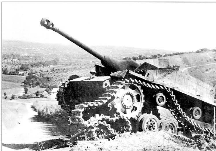
An American soldier sits on a knocked out StuG.III Ausf.G. It features the waffle pattern Zimmerit coating applied at the Alkett plant between September 1943 and September 1944. It is also fitted with the 'topfblende' cast gun mantlet and the shot deflector in front of the commander's cupola. Steel return rollers were introduced in November 1943, however rubber tired rollers continued in use until stocks were used up.
