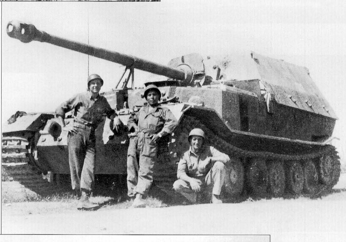
Three American soldiers pose in front of a captured Elephant from s.Pz.Jg.Abt.653 that broke down and had to be abandoned in late May 1944. The vehicle is finished in a camouflage scheme of green and brown patches applied over the dark yellow base color and a three digit tactical number, '102', has been painted in white on both sides. Not visible is the gothic script letter 'U', an abbreviation for 1.Kompanie commander Hauptmann Helmut Ulbricht, also painted in white on the upper right side of the upper rear plate.
