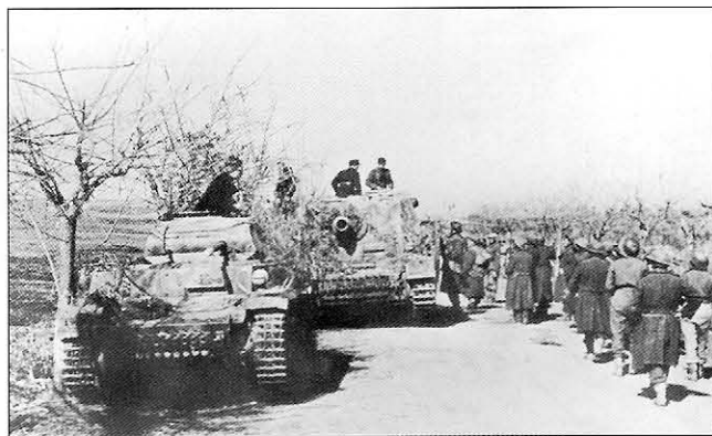
Sturmpanzer-Abteilung 216 was also one of the units rushed to the Anzio-Nettuno area in February 1944. They were the first unit to be equipped with the Sturmpanzer IV, which was first successfully employed at Kursk in July 1943. This one is a mid production vehicle built on a Pz.Kpfw.IV Ausf.H chassis and still has the sliding driver's visor similar to the Tiger I. In front, is an obsolete Pz.Kpfw.II Ausf.A-C, probably in use as a command vehicle. A column of British POW's can be seen marching to the rear along the right side of the road.
