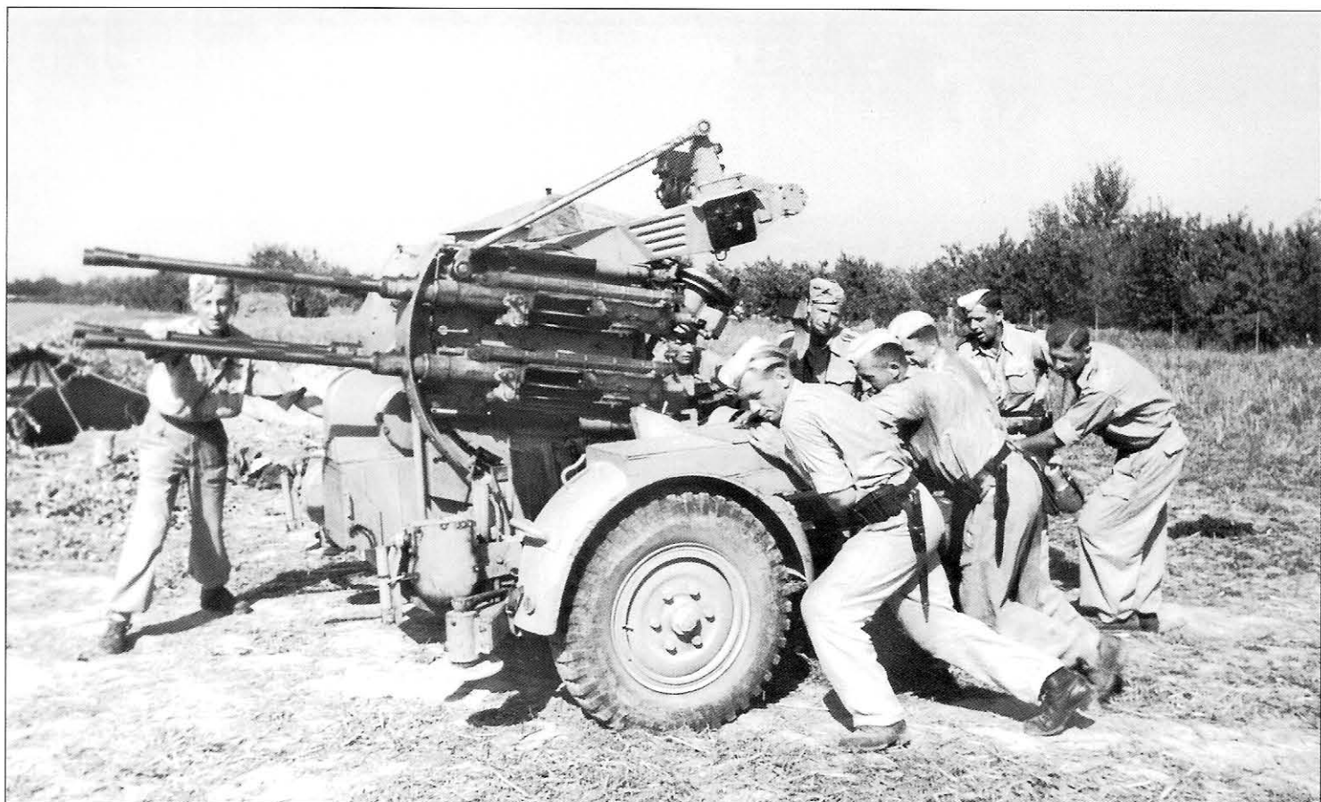
A 2cm Flakvierling 38 anti-aircraft gun is moved into position by its crew. All branches of the German Armed Forces used this gun and by August 1944, the Luftwaffe alone had around 3600 in service. It was capable of firing at 880 rpm and had a maximum effective ceiling of 2200 m.
