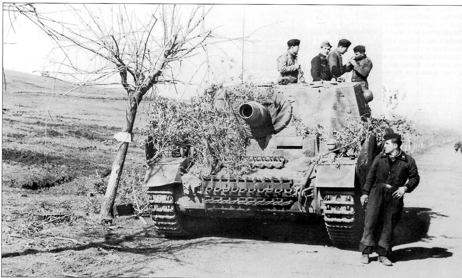
The same Sturmpanzer IV with the column of British POW's receding in the distance. It is finished in overall dark yellow with random patches of brown camouflage paint and is fitted with a canvas collar around the mantlet. The crewman standing on the ground is wearing a pair of field grey coveralls over his black Panzer uniform and has the lapels of his Panzer jacket pulled out.
