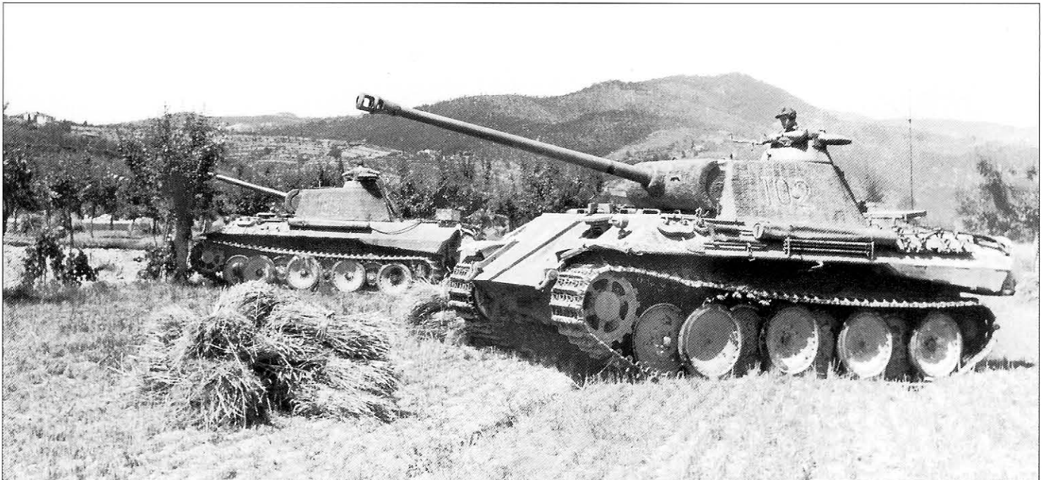
Two Panzerbefehlswagen V Panther Ausf.A from I./Pz.Rgt.4 near Florence during the summer of 1944. They are both early Ausf.A with the 'letterbox' machine gun port on the glacis. The one in front, tactical number '102', is a purpose built Befehls-Panther and is fitted with an armored mount for the star antenna on the engine deck and has the spare antenna storage tubes mounted below the gun cleaning rod storage tube. The one behind with tactical number '113', is a standard gun tank that has been assigned as a staff vehicle. Both Panthers are painted overall dark yellow with red tactical numbers outlined in white.
