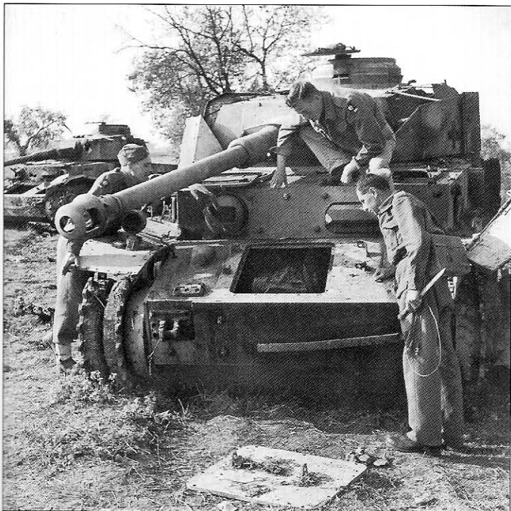
Three British soldiers from the 78th Infantry Division examine a knocked out Pz.Kpfw.IV Ausf.G near San Salvo on the Adriatic coast in November 1943. It has been fitted with additional 30mm armor plates that have been bolted to the superstructure front and welded to the hull front. The meaning of the small cross, visible to the left of the driver's visor, is unknown and other photos show that it was applied at the factory. The missing tracks have exposed the curved armor shield that protected the final drive housings on the Pz.Kpfw.IV Ausf.B to G. Reinforced final drive housings were installed on the Pz.Kpfw.IV Ausf.H replacing the curved shield. Note how mud has built up around the drive sprocket. The soldier in front is carrying a German field telephone slung over his shoulder.
