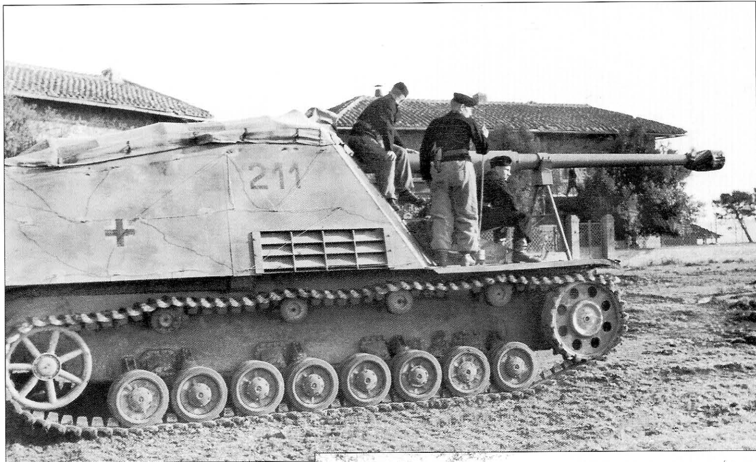
A Nashorn from 2./s.H.Pz.Jg.Abt.525 in the Anzio-Nettuno area in March 1944. This is an early production vehicle fitted with the early eight-hole drive sprocket with a spacer ring to accommodate the 40cm wide track. It is painted in overall dark yellow with a camouflage scheme of green and brown patches. Markings include the standard Balkenkreuz along with a black three digit tactical number, '211', painted on the side. The tactical number is also repeated on the left side of the gunshield. The unit emblem, consisting of a crouching lion perched on top of a tracked chassis, was painted on the left hinged mudguard. Additional tie downs have been welded on the sides to hold wire for attaching foliage for camouflage.
