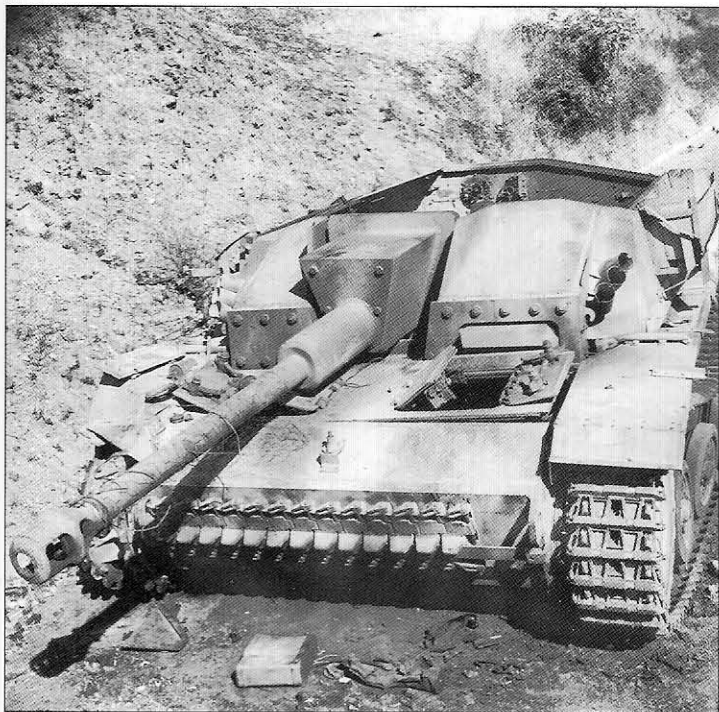
A StuG.III Ausf.G sits alongside a road near Satriano di Lucania, southwest of Potenza in September 1943. The roof of the fighting compartment has been completely blown off as a result of an internal ammunition explosion. It is finished in overall dark yellow with a camouflage scheme of green patches. No unit markings are visible but both 16.Panzer-Division and 29.Panzer-Grenadier-Division were operating in the area and both were equipped with StuG.III.
