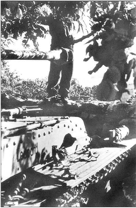
An early Marder III Ausf.M sits in a hull down position behind a stone fence while one of the crew keeps a watchful eye on the ground in front with his binoculars. The name 'Leopard' can be seen painted in black on the right side of the hull behind the driver's compartment. The early Marder III was fitted with a rounded, cast cover on the driver's compartment. A redesigned welded cover was introduced at the end of 1943.
