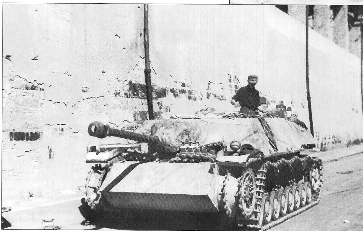
A damaged early Jagdpanzer IV awaits a recovery vehicle to tow it to the workshops. The transmission has probably seized up and so both tracks have been shortened and linked together bypassing the drive sprocket. The early Jagdpanzer IV mounted the 7.5cm PaK39/L48 gun, some of which were fitted with a muzzle brake like this one. From January to November 1944, a total of 769 of these purpose built Panzerjäger were built and saw their first action with Panzer-Division 'Hermann Göring' in the spring of 1944.
