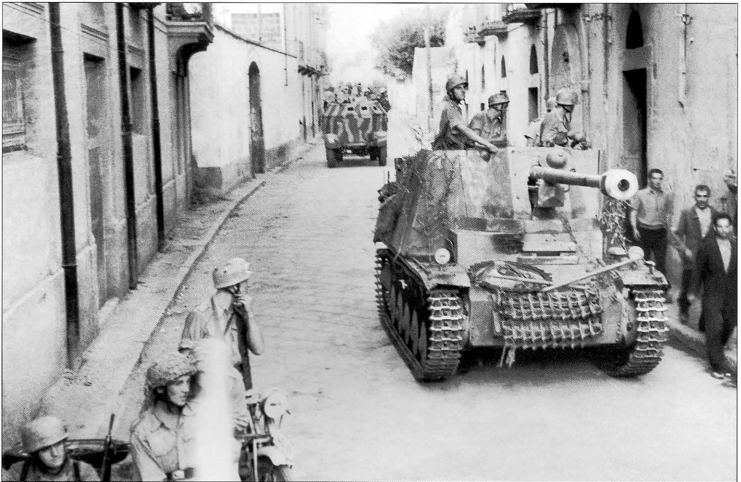
Another Marder II self-propelled anti-tank gun of Panzer-Artillerie-Regiment 'Hermann Göring' passing through an Italian village followed by a 2cm Flakvierling 38 auf schwerer Geländegängiger Lastkraftwagen 4.5t. More simply put, this was a 2cm Flakvierling 38 mounted on the chassis of the Mercedes-Benz L4500 4.5 ton truck. The driver's cab and radiator received light armor plating and the rear deck was fitted with folding sides to increase the platform size. It also carries a striking hard-edged camouflage scheme of green stripes over the dark yellow base.
