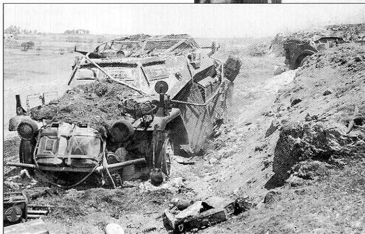
An Sd.Kfz.223 leichte Panzerspähwagen (Fu) of Panzer-Division 'Hermann Göring' in the Vizzini area along the route taken by the 1st Canadian Division. An internal explosion has scattered debris around the vehicle and dislodged the frame antenna.
