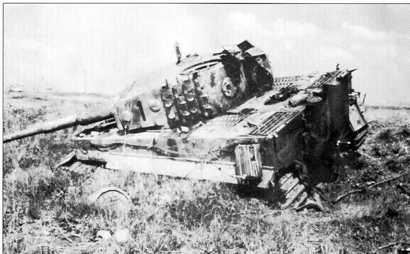
One of the early Tiger I Ausf.E originally from s.Pz.Kp. 'Meyer' destroyed during the battle near Cisterna 25 May 1944. The Tigers had been repainted with a camouflage scheme of green and brown over the dark yellow base color and had new tactical numbers from '1', seen here, to '8'. Note the early cupola lying on the ground after being blown off by an internal explosion. On 3 March 1944, the remaining Tigers in the Kompanie were integrated with s.Pz.Abt.508. Hidden from view, on the other side of the road, was an overturned Elephant from s.Pz.Jg.Abt.653.
