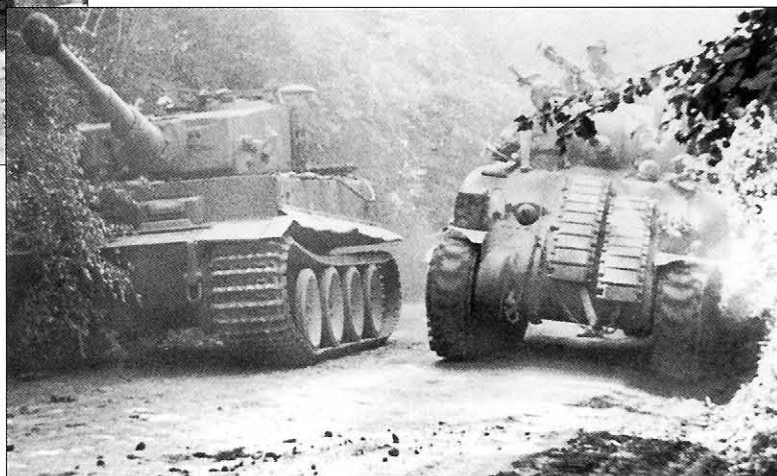
An early M4A1 Sherman winds its way past several abandoned German vehicles including this mid-production Tiger I from s.Pz.Abt.508. There is no visible damage on the Tiger and it is likely that it was simply abandoned after it broke down. Note the dust cover still in place on the muzzle brake and the gun locked in the traveling position.
