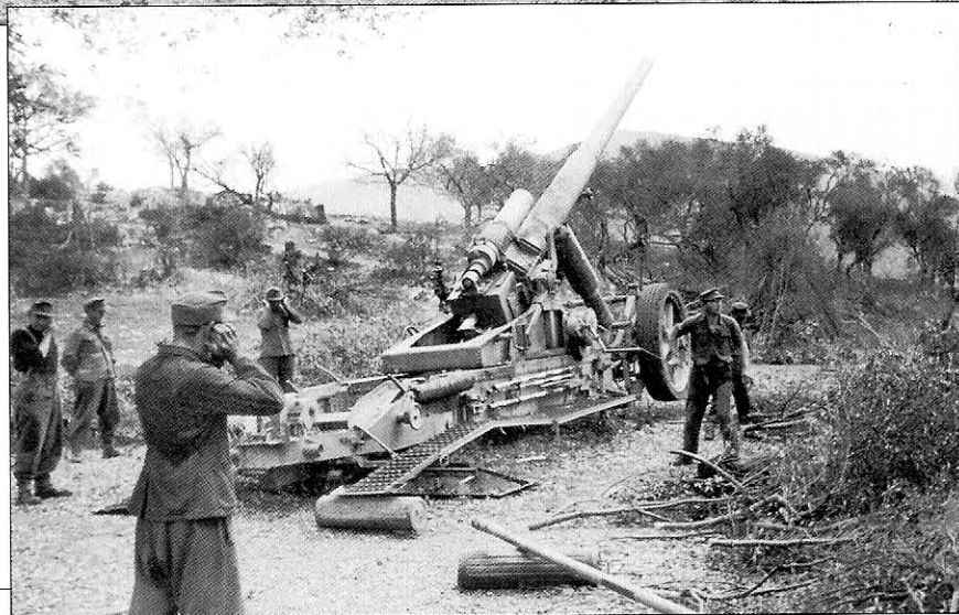
A 17cm Kanone 18 in Morserlafette fires on the Allied beachhead at Anzio. This heavy artillery piece could fire a 68kg high explosive projectile to a maximum range of 29600m. It was mounted on a carriage that not only had a gun recoil system but the gun platform slid back on the trails providing a second recoil system. In action, the whole carriage was mounted on a turntable that provided a complete 360° rotation. The gun was normally towed by the Sd.Kfz.8 half-track prime-mover.
