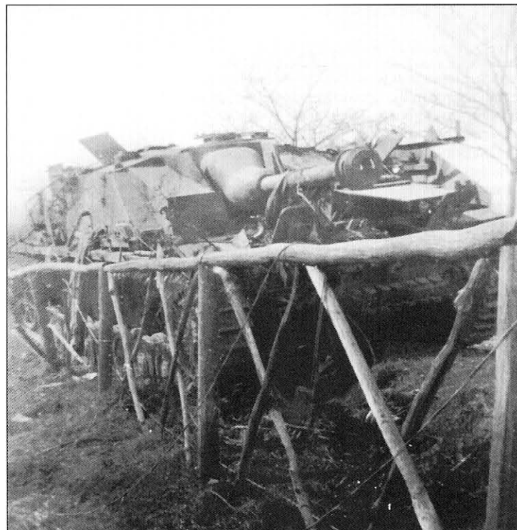
Another view of the same StuG.IV showing an additional armor plate hinged in front of the driver's position. Here, the opened access hatch on the glacis is holding up the plate. 34.Infanterie-Division surrendered their remaining vehicles at Ivrea, north of Torino, on 5 May 1945. Photos taken at that time show their vehicles fitted with similar additional armor.
