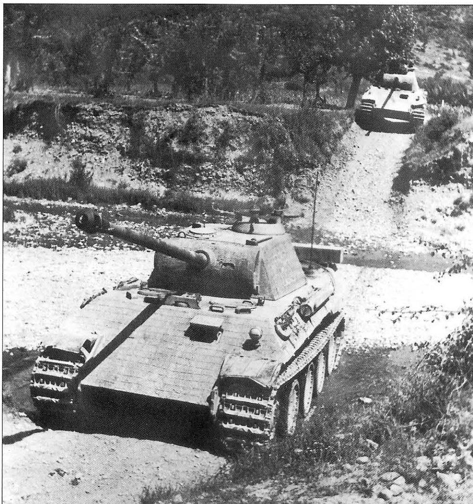
Befehls-Panther '113' shown crossing a small stream with '102' following behind. The early Panther Ausf.A was equipped with the T.Z.F.12 binocular gunsight until mid-November 1943, when the T.Z.F.12a monocular gunsight was introduced.
