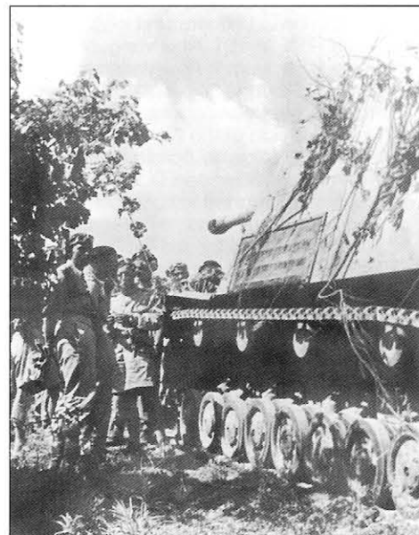
A Nashorn from s.H.Pz.Jg.Abt.525 is inspected by several British Commonwealth troops in the late spring of 1945. It has been fitted with a screen over the engine air intake to prevent debris from being sucked into the engine compartment. On 9 September 1944, 1./s.H.Pz.Jg.Abt.525 was ordered back to Germany to re-equip with the Jagdpanther, while 2./525 and 3./525 remained in Italy, surrendering to American forces on the Po River at the end of the war.
