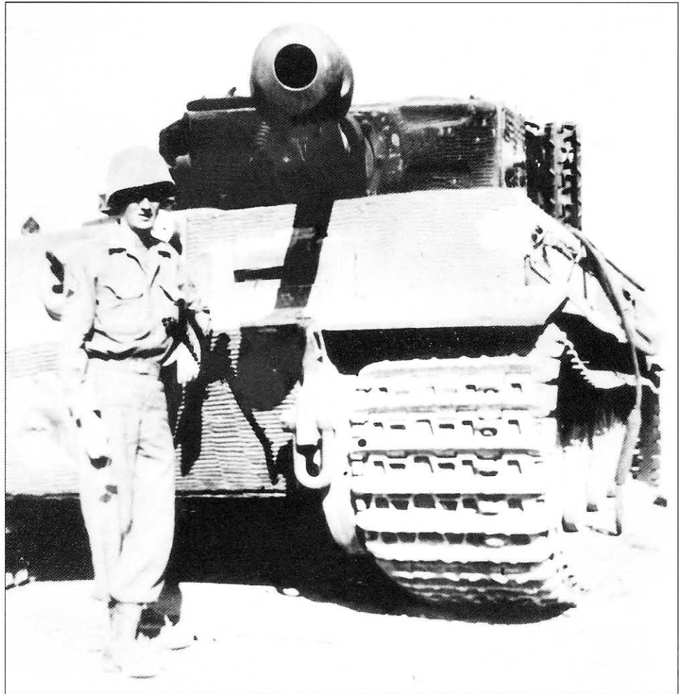
A soldier from the U.S. 133rd Infantry Division poses in front of a knocked out late Tiger I Ausf.E from s.Pz.Abt.508 in the Cecina region in July 1944. The impact point from a round that did not penetrate the 100mm thick lower hull plate can be seen to the left. This Tiger I was hit by a 75mm round into the engine compartment through the thinner, 80mm side hull plate resulting in an engine fire that destroyed the vehicle.
