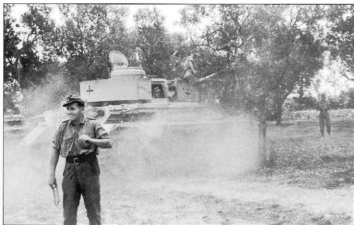
A Pz.Kpfw.IV Ausf.G from the same unit raises a great cloud of dust as it moves into position among the grove of olive trees. Both vehicles are fitted with the 'Filzbalgfilter' engine air filter system on the right mudguard introduced in May 1943. The officer standing in front is wearing the Iron Cross First Class pinned to the left breast of his tropical shirt.
