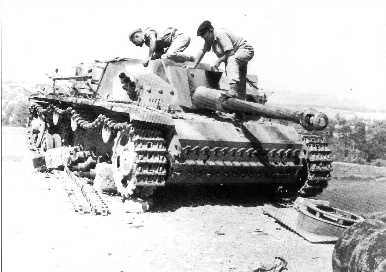
An early StuG.III Ausf.G is inspected by two British soldiers in the summer of 1944. It is fitted with the smoke grenade launchers that were installed on vehicles manufactured from February to May of 1943 and has the retrofitted Schürzen brackets that were installed by field workshops beginning in early June 1943. The chassis number '92271' is painted on the 30mm supplementary armor plate on the right side of the vehicle.
