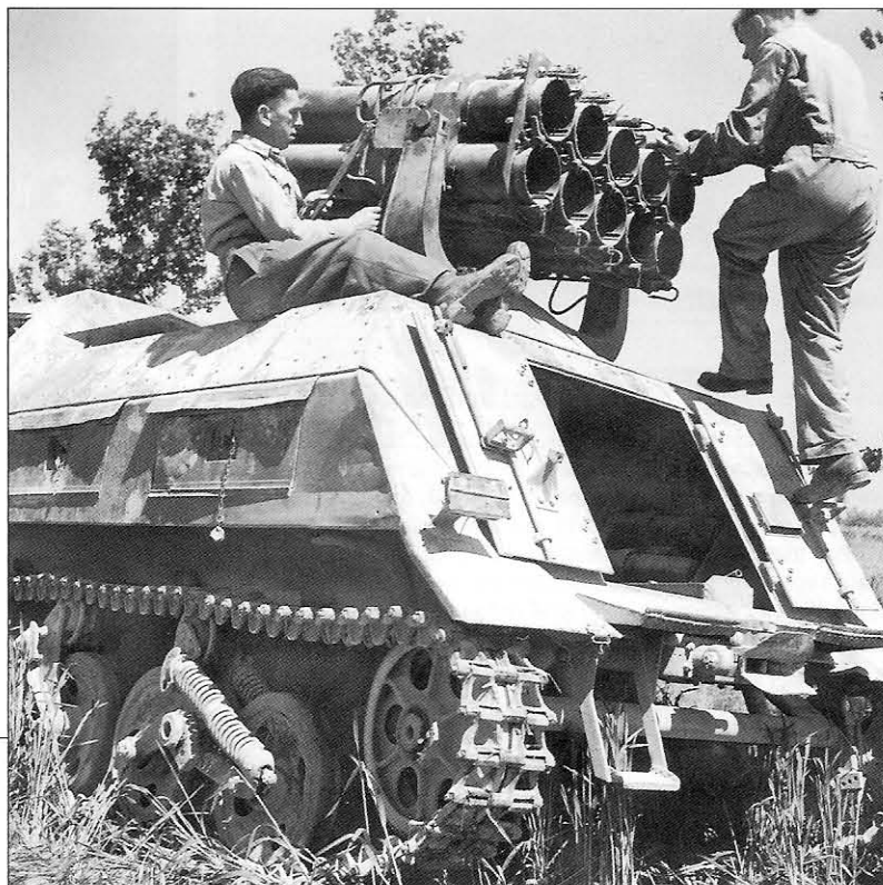
Two Commonwealth soldiers examine an abandoned 15cm Panzerwerfer 42 (Sd.Kfz.4/1). The two men are probably British judging from the style of hobnail boots on the man on the left and the small bandage pocket visible on his battledress trousers. There were 300 Panzerwerfer 42 built from April 1943 to March 1944 plus another 19 converted from Munitionskraftwagen für Nebelwerfer in June 1944.
