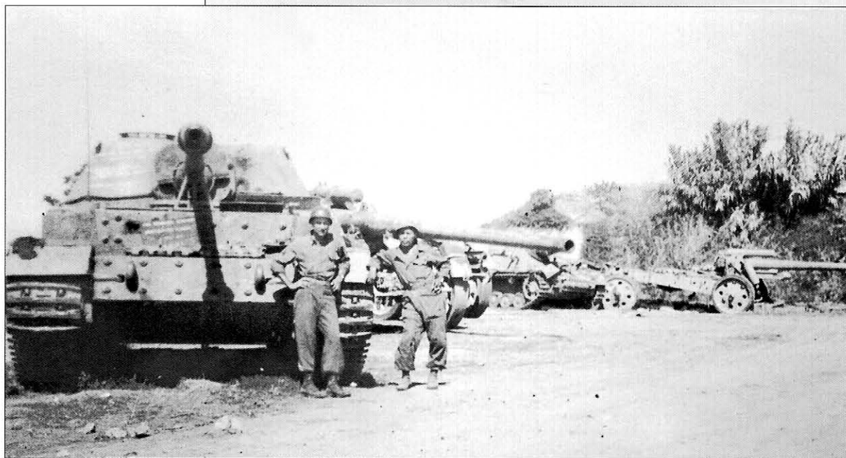
Another photo of the same Elephant from s.Pz.Jg.Abt.653 at an enemy vehicle collection point. In the background can be seen a Sturmpanzer IV from Sturmpanzer-Abteilung 216 along with two large artillery pieces, a 15cm K18 on the left and a schwere 10cm K18 on the right. This Elephant was shipped back to Aberdeen Proving Grounds in the U.S. where it can still be seen today.
